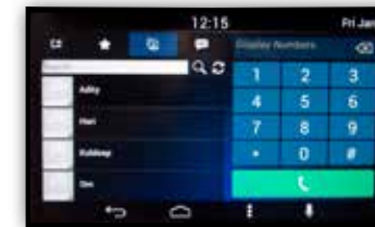
NAV+ HD integrates Bluetooth wireless technology with an in-cab microphone and speaker. Just pair it with your compatible Bluetooth phone and talk hands-free.
