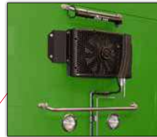
The remote condenser with brushless fan assembly is installed centrally on the upper exterior wall for optimum performance.
