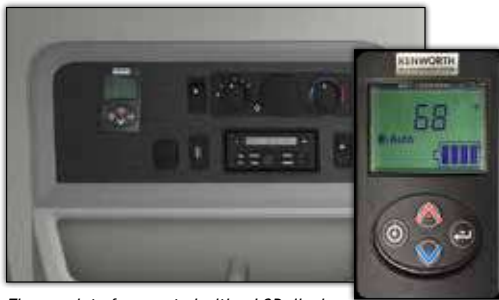
The user interface control with a LCD display conveniently located on the sleeper control panel provides automatic temperature control in both A/C and Heating modes.
