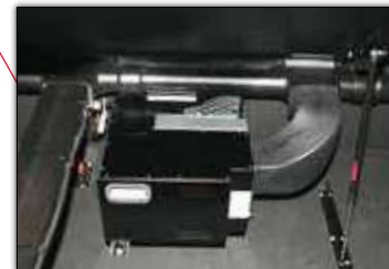
The compact brushless DC compressor and evaporator assembly is strategically located in the sleeper storage area.
